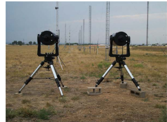
Figure 2: The two 14-inch telescopes, spaced laterally by 2.0 m and pointing at two test-light arrays, which were also laterally spaced by 2.0 m and 174 m away from the telescopes. The propagation paths were horizontal and 1.7 m above flat ground.
