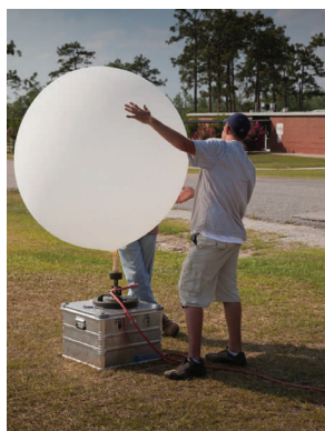
Kenneth Pratt inflates a research weather balloon in preparation for launch with a radiosonde.
